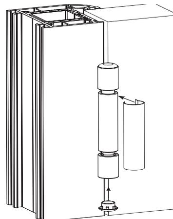
Replace the lower cap and the cover cap
