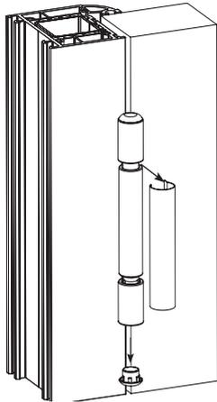
Remove the lower cap and the cover cap.
