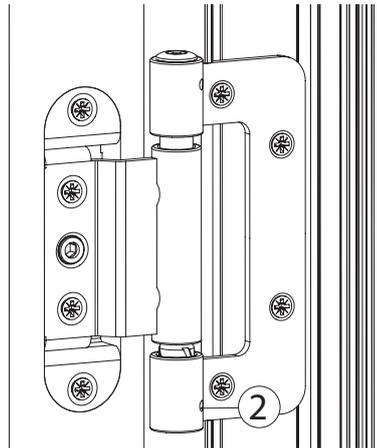
Open the door and unscrew but do not fully remove the lower security screw marked 2.
