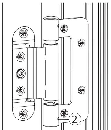
Open the door and tighten the lower security screw marked 2.
